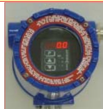
EZR-M Microprocessor Based Electronics feature 2 programmable relays 4-20mA output and LED Display
